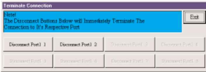
Figure 7-3. Terminate Connection screen.
