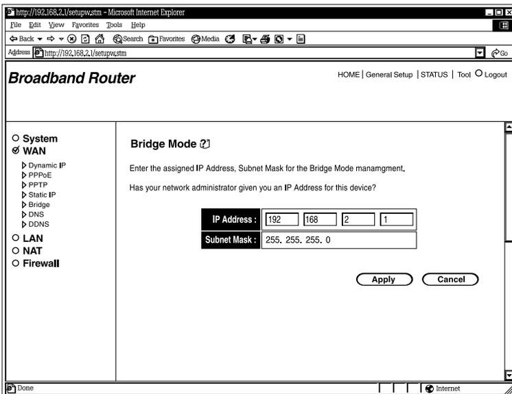
Figure 5-8. Configuring the router as a bridge.
