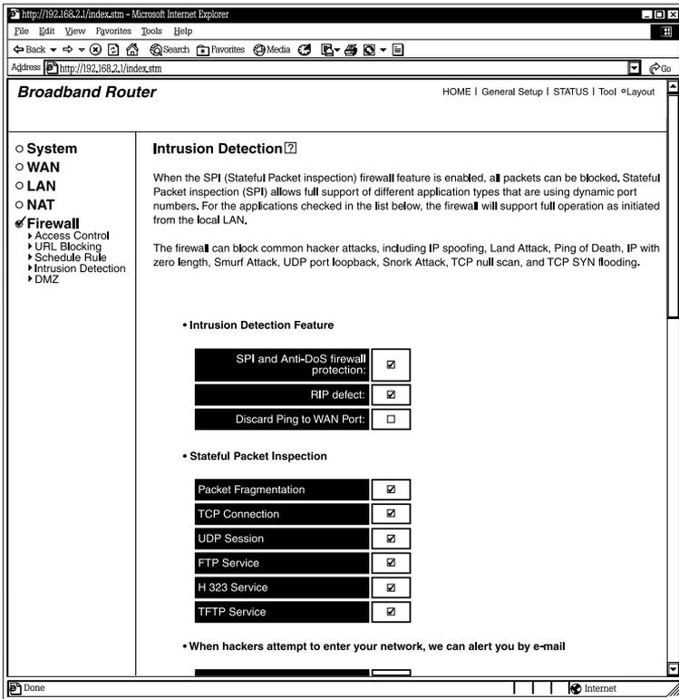
**Figure 5-29. Intrusion Detection screen, part #1.**
