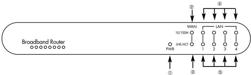
**Figure 2-2. Front-panel LEDs.**
