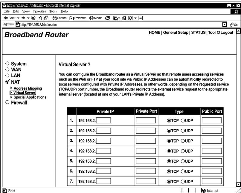
**Figure 5-19. Configuring the router as a virtual server.**
