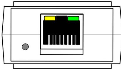
Figure 4. LED Indicators on the LPD401A
