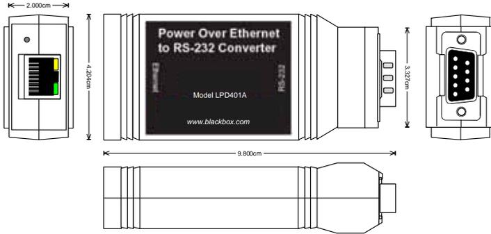
Figure 19. Dimensional Diagram of the LPD401A
