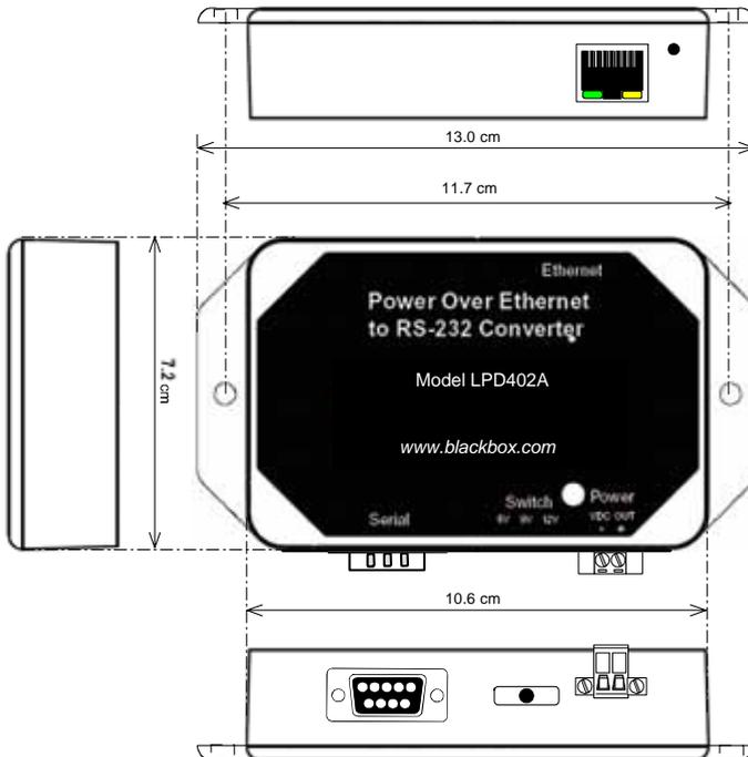
Figure 20. Dimensional Diagram of the LPD402A
