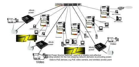
Example 4b. LP004A (Power Source Switch) for PoE device only
