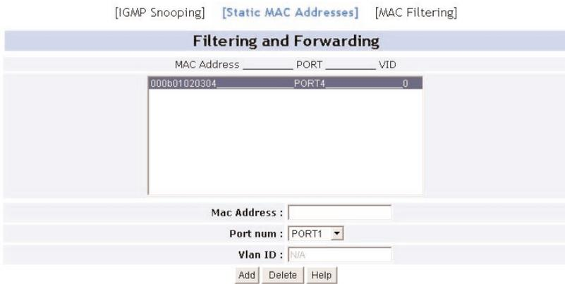
Static addresses currently defined on the switch are listed below. Click Add to add a new static entry to the address table.
