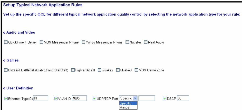
**Fig. 3-51 Set up Typical Network Application Rules**
