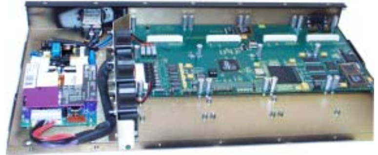
Figure 3.5.1b: LE2425A Managed fiber switch, Top view without chassis cover
