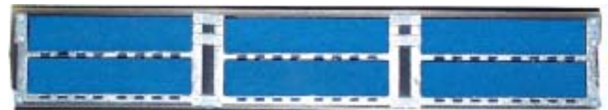
Fig. 3.5.2h Inside view of chassis cover (from the rear), showing the front panel screen plates installed inside the chassis cover using brackets and screws
