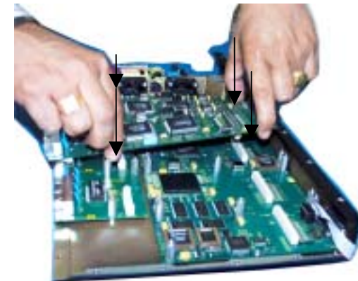
Figure 3.5.3a: Top View - 6 retaining screws shown by arrows
