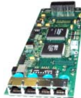
Fig. 3.5.2c Daughter Board, top view of version for 4 copper 10/100 ports
