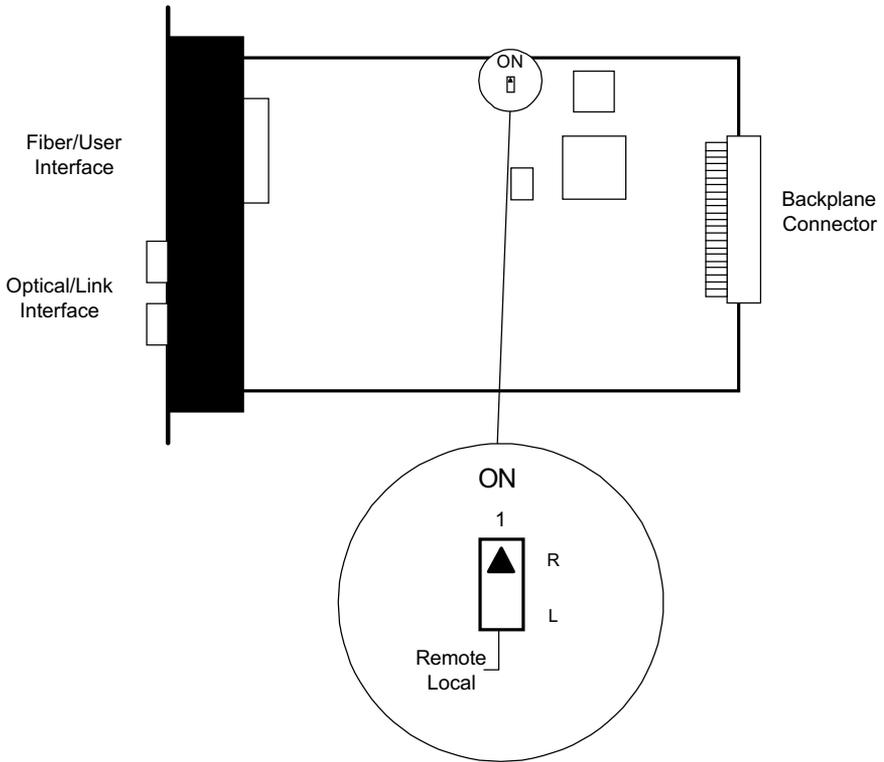
Figure 4 - Switch Position
