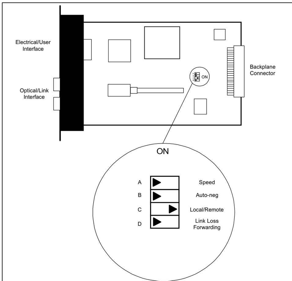
Figure 3 - Switch Positions
