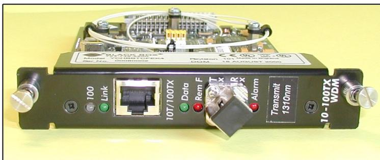
Figure 1 - CityLIGHT 10/100 Ethernet WDM Transceiver Card
