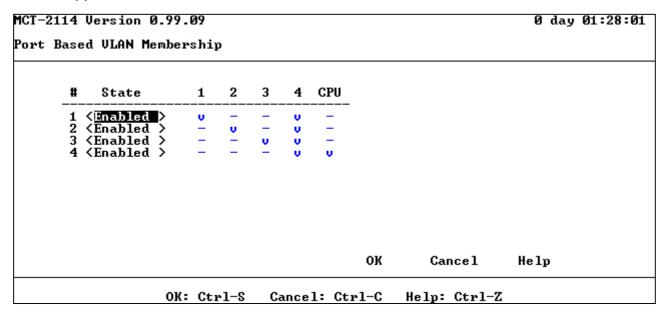
The converter switch supports 4 Port Based VLAN.
