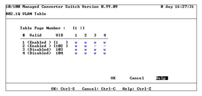
The converter switch supports 16 802.1Q VLAN.
