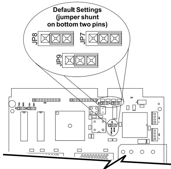
**Figure 2.4 Factory Configured Jumpers**
