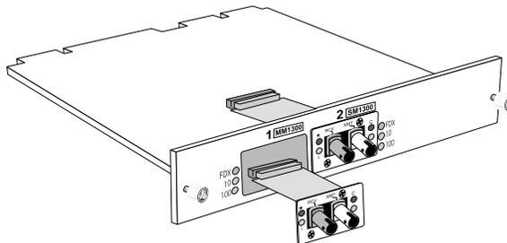
**Figure 2.2 Installing a 100-Mbps Module**
