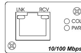
**Figure 2.7 100-Mbps Module, TX**
