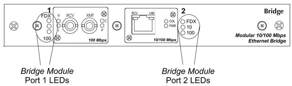
**Figure 2.6 Bridge Module LEDs**
