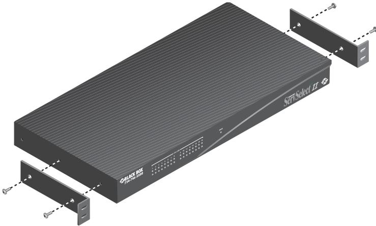
**Figure 3-1. ServSelect II Horizontal Installation**
