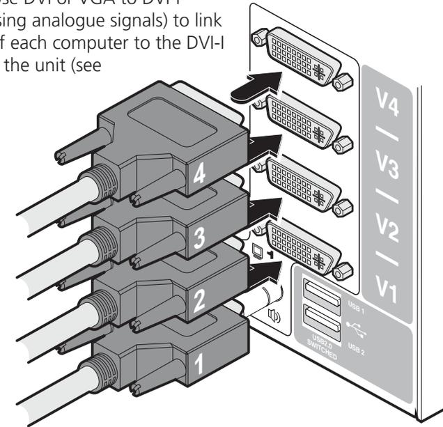
*Note:* On the rear panel of the unit, connectors belonging to the same channel are stacked vertically. The connectors at each horizontal level (V1 to V4) will be switched through to the user console DVI-I connector which is at the same level:
