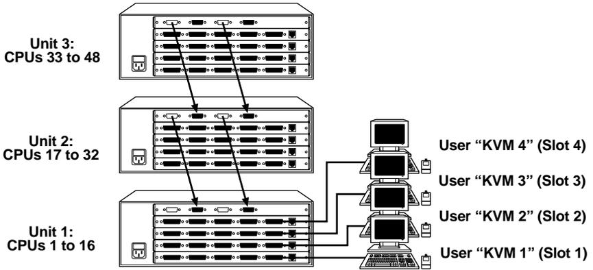
Figure 3-5. 4-User models in a regular bus topology.
