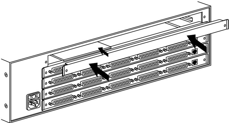
**Figure E-2. Installing a Terminator Card.**
