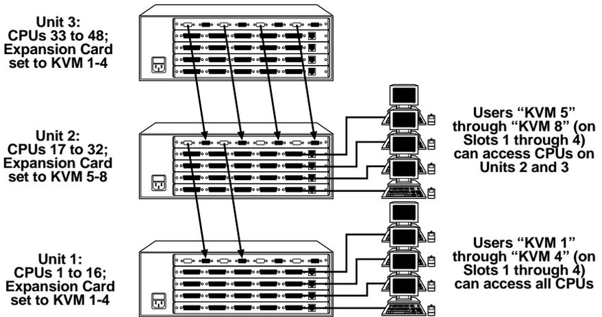
Figure 3-6. 8-User models in a regular bus topology.
