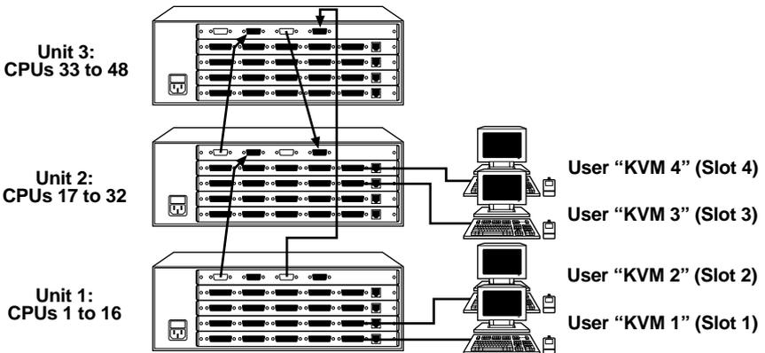
Figure 3-8. 4-User models in a carefully cabled custom split-bus topology.
