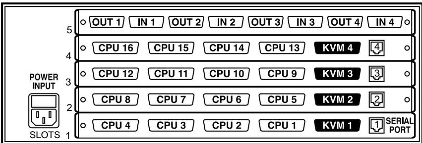
**Figure 2-3. A fully populated 8-User rear panel, numbering shown. (For clarity, Expansion-Card connectors are shown disproportionately large.)**
