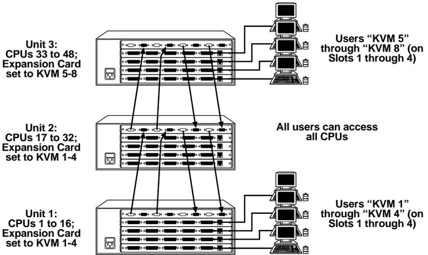
Figure 3-9. 8-User models in a standard split-bus topology.
