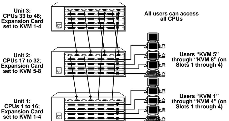
Figure 3-10. 8-User models in a carefully cabled custom split-bus topology.
