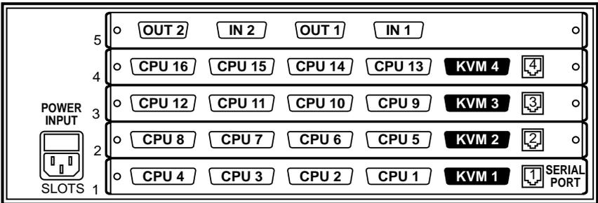
**Figure 2-2. The same rear panel, slot and port numbering shown.**
