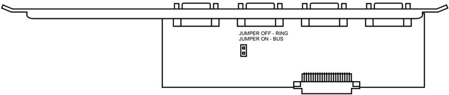
**Figure E-3. The RING/BUS jumper.**
