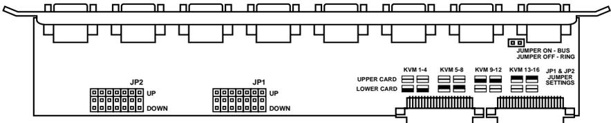
**Figure 3-4. The jumpers on the 8-Port Expansion Card.**
