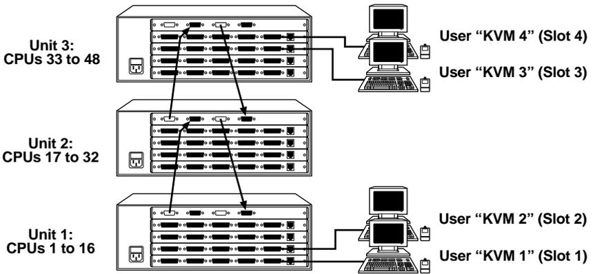
Figure 3-7. 4-User models in a standard split-bus topology.
