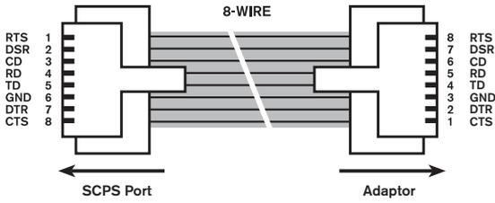
**Figure 8-1. 8-wire RJ45 Reversing Cable**
