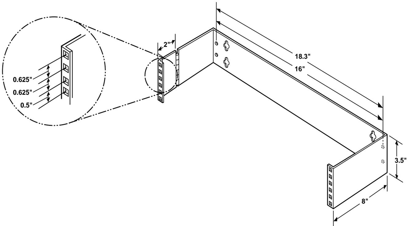
Figure 3. Size Specifications for the Wall Mount Patch Bracket-2 (JPM082).
