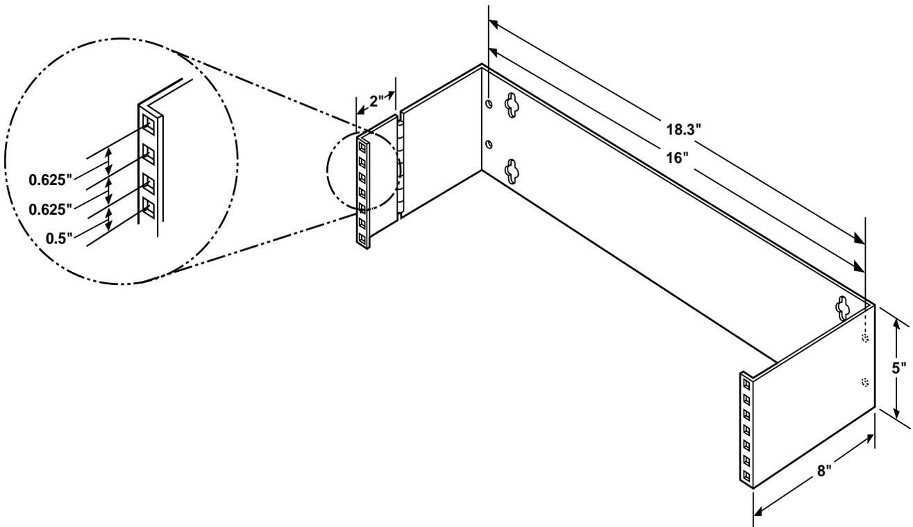
Figure 2. Size Specifications for the Wall Mount Patch Bracket-3 (JPM081).
