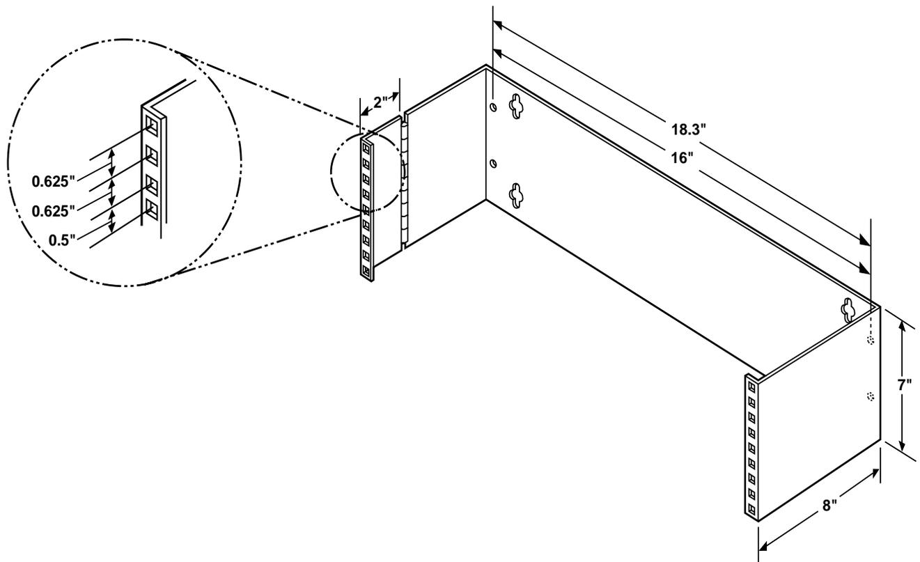
Figure 1. Size Specifications for the Wall Mount Patch Bracket-4 (JPM080).
