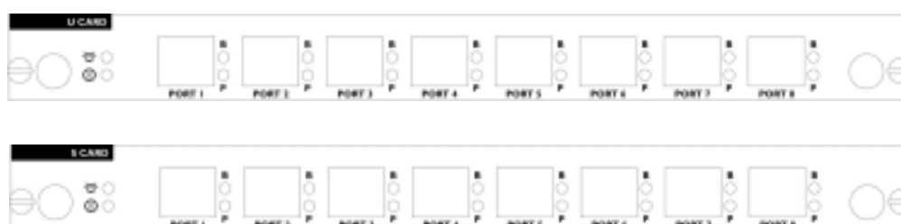
Figure 3 The Primary to Basic Rate ISDN Multiplexer U card and S card
