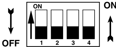
Figure 3-5. Closeup of the DIP switches.
