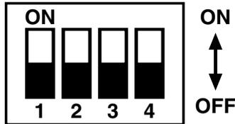
**Figure 3-10. Closeup of the DIP switches.**
