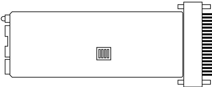
**Figure 3-9. Switch S1 (located on the bottom of the IC701A’s PC board).**
