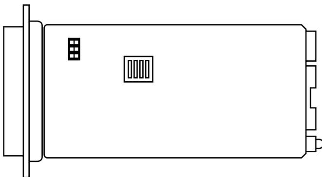
**Figure 3-7. Straps JP1 and JP2 (on the bottom of the IC700A’s PC board).**
