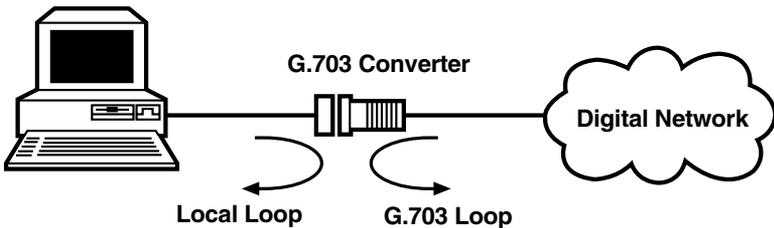
Figure 5-2. Test mode operation: Local loop/G.703 loop.
