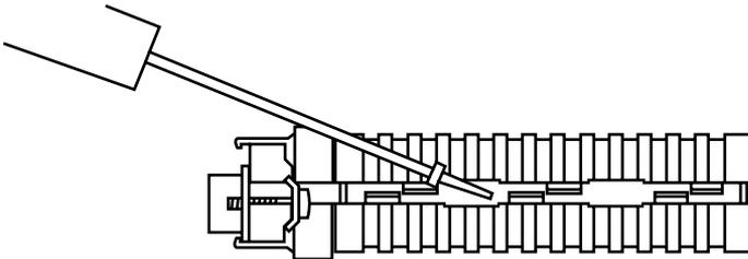
**Figure 3-4. Using the screwdriver to open the main part of the IC701A's case.**
