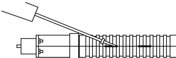
**Figure 3-1.** Using the screwdriver to pry open the IC700A or IC702A's case.
