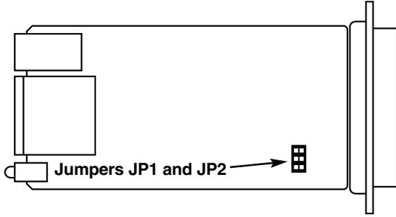
**Figure 3-16. (JP1 and JP2 on the top of the IC702A’s PC board).**
