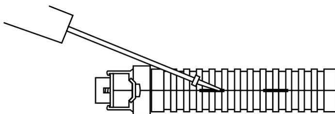
**Figure 3-2.** Using the screwdriver to pry open the IC701A's case.
