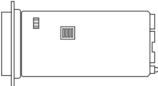
**Figure 3-5. Switch S1 (located on the bottom of the IC700A’s PC board).**
