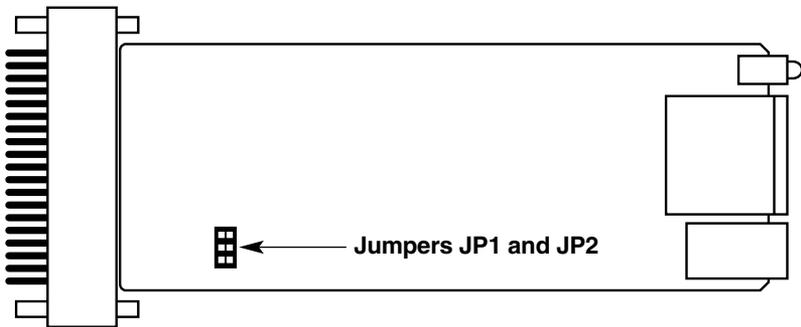
Figure 3-12. JP1 and JP2 (on the top of the IC701A’s PC board), as seen when the V.35 connector shroud is removed.
