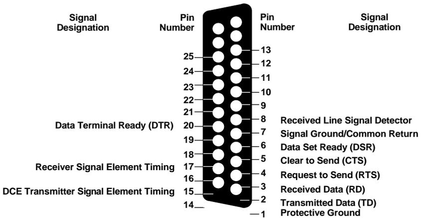
**Fig. A-2. The RS-232 Interface (female) asynchronous DCE**
