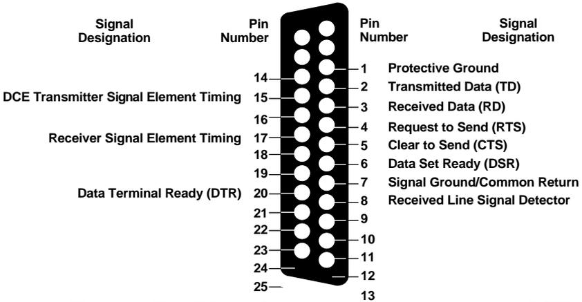
**Fig. A-1. The RS-232 Interface (male) synchronous DTE**
