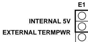
Figure 5-3. Terminator Power Jumper Locations.
