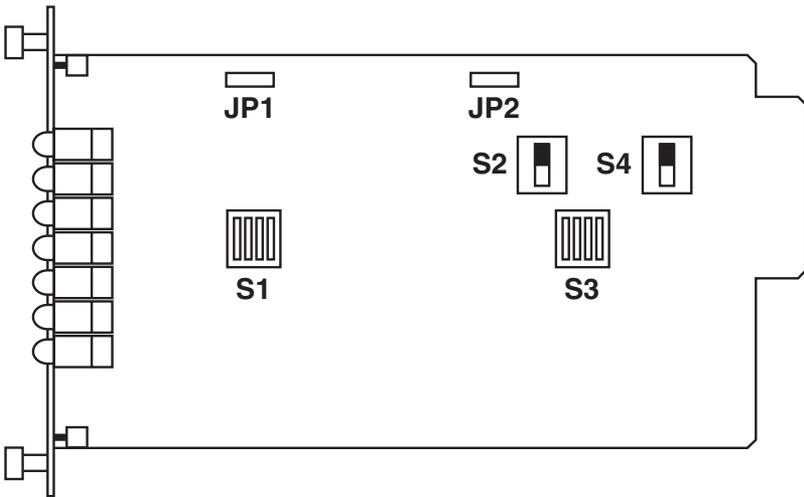
**Figure 3-1. Location of configuration switches and jumpers on the Async 232↔422/485 Card board.**
