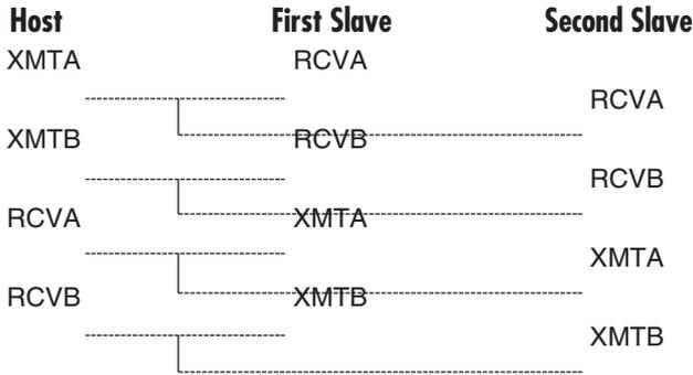
**Figure 4-3. Star wiring for the Async 232↔422/485 Card host and slaves.**
