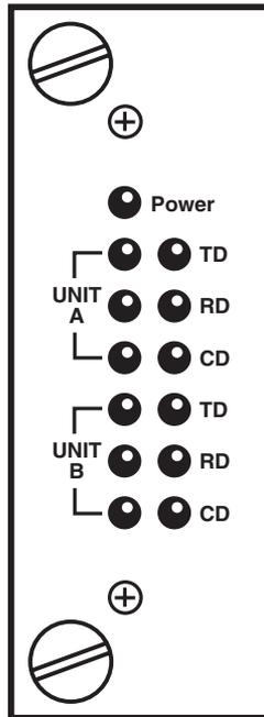
**Figure 5-1. The Async 232↔422/485 Card front panel, showing LED positions.**
