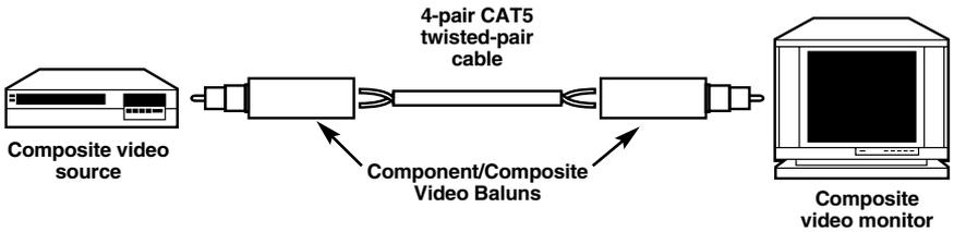
Figure 3-3. Composite video connection.
