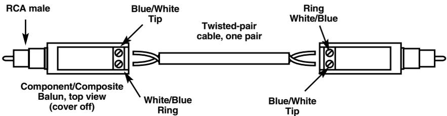
Figure 3-1. The balun's wiring configuration.
