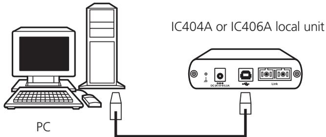
NOTE: The power adapter is not required at the local unit for normal operation.
