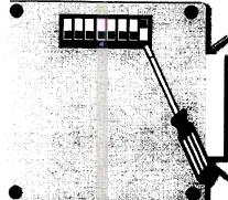
Switch operations:- To set the configuration switches use a small instrument such as a screwdriver. The example on the left shows switch 8 in the ON position and switches 1 to 7 in the OFF position.
