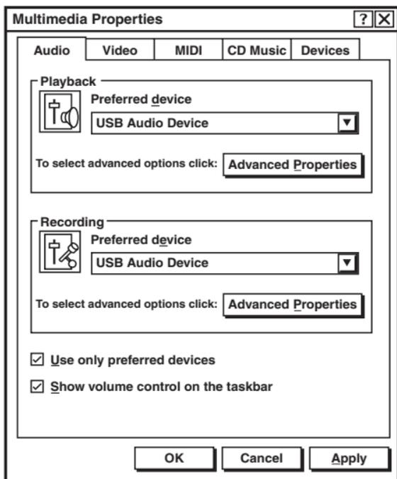
Figure 4-2. Selecting the USB Audio Device screen.
