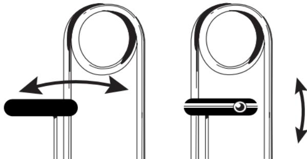
The on-line indicator snaps conveniently onto the headset stand.
