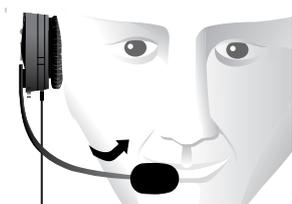
**Figure 4-5. Adjusting the Microphone Boom.**
