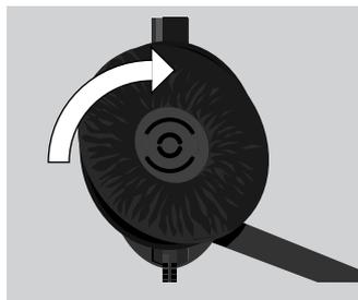
Figure 3-12. Replacing the Earplate and Ear Cushion.
