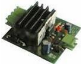
The 12V DC Power Supply PCB with all components assembled.
