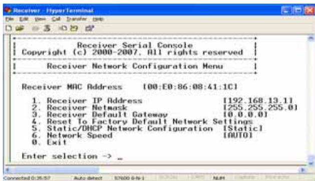
**Figure 4-17. Receiver Network Configuration Menu (Extender and Matrix Mode)**
