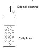
Fasten the rubber antenna (which is the 1-ft. adapter cable that's included in drive kit) to where the original antenna was on the cell phone.
