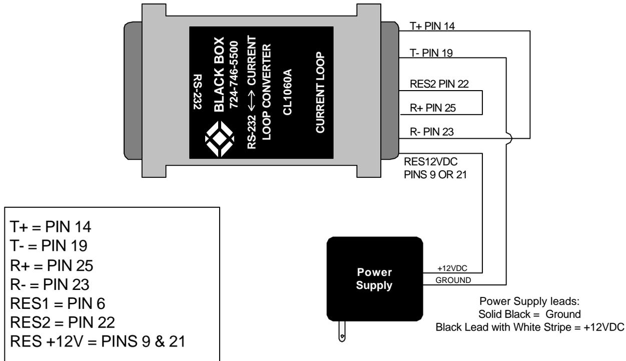
CL1060A can be ordered with a male or female DB25 Current Loop connector. The RS-232 connector is only DB25 female.
