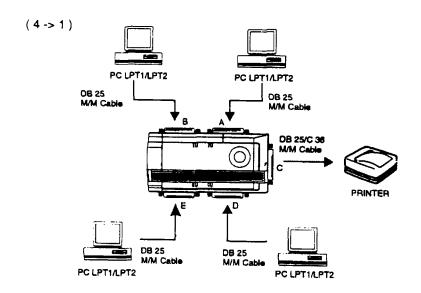
Fig. A 4-IN- 1 -OUT configuration
