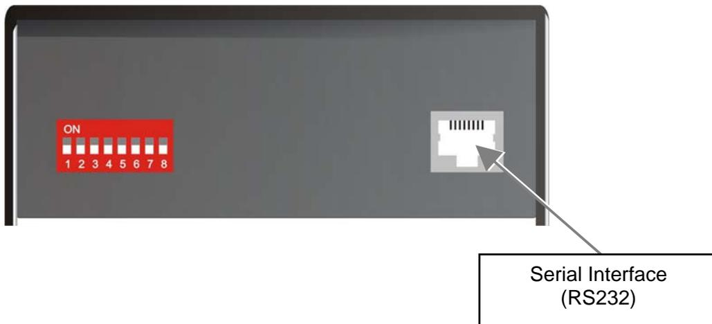
You can find the allocation of the serial interface under **Serial Interface** on page 116. A standard cable RJ45 on DB9 to a CPU is included in delivery.
