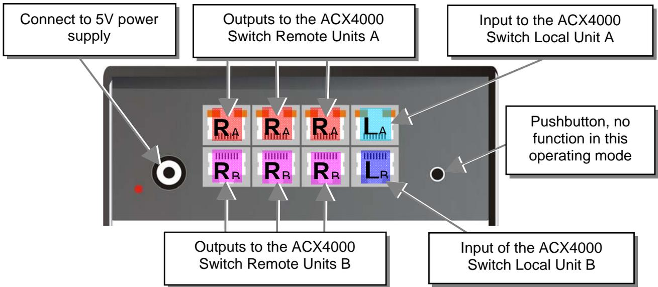
Two different signals from two Local Units are each distributed to 3 outputs and transferred over CATx- cables to 3 Remote Units. Using a second stage of Multiplex Repeater up to 2x9 (2x21) monitors can be supplied with video (and optionally audio).
