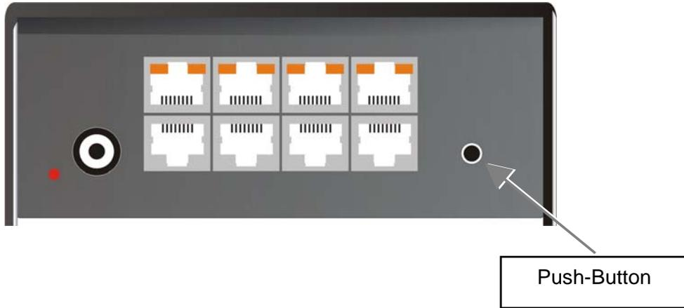
The device switches to the next channel with each key press. The changeover will only be executed if the push-button is not operated for longer than 2 seconds. With each key press, the display will switch to the next channel indicated by a rapidly blinking LED. If the last channel is reached, the device will switch to the first channel.
