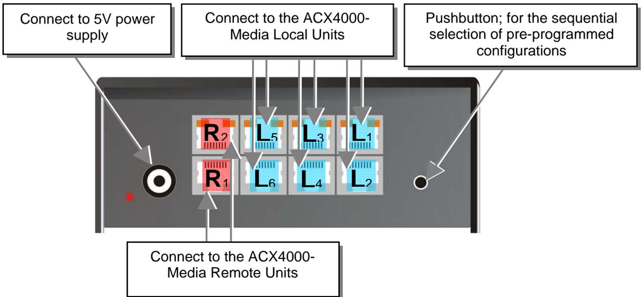
The signals of 6 Local Units can be switched on up to 2 outputs (also on several) and be transferred over CATx- cables on up to 2 Remote Units. Optionally a further ACX4000 Switch can be inserted for a second switching stage.
