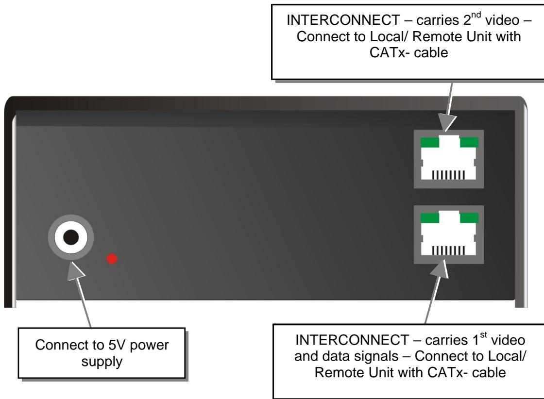
**ACX4000- KVM Dual head, Local/ Remote Unit, with optional audio – rear view**
