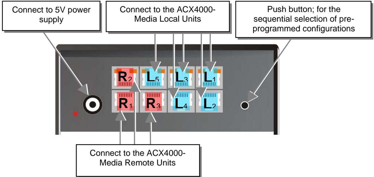
The signals of 5 Local Units can be switched on up to 3 outputs (also on several) and be transferred over CATx- cables on up to 3 Remote Units. Optionally a further ACX4000 Switch can be inserted for a second switching stage.
