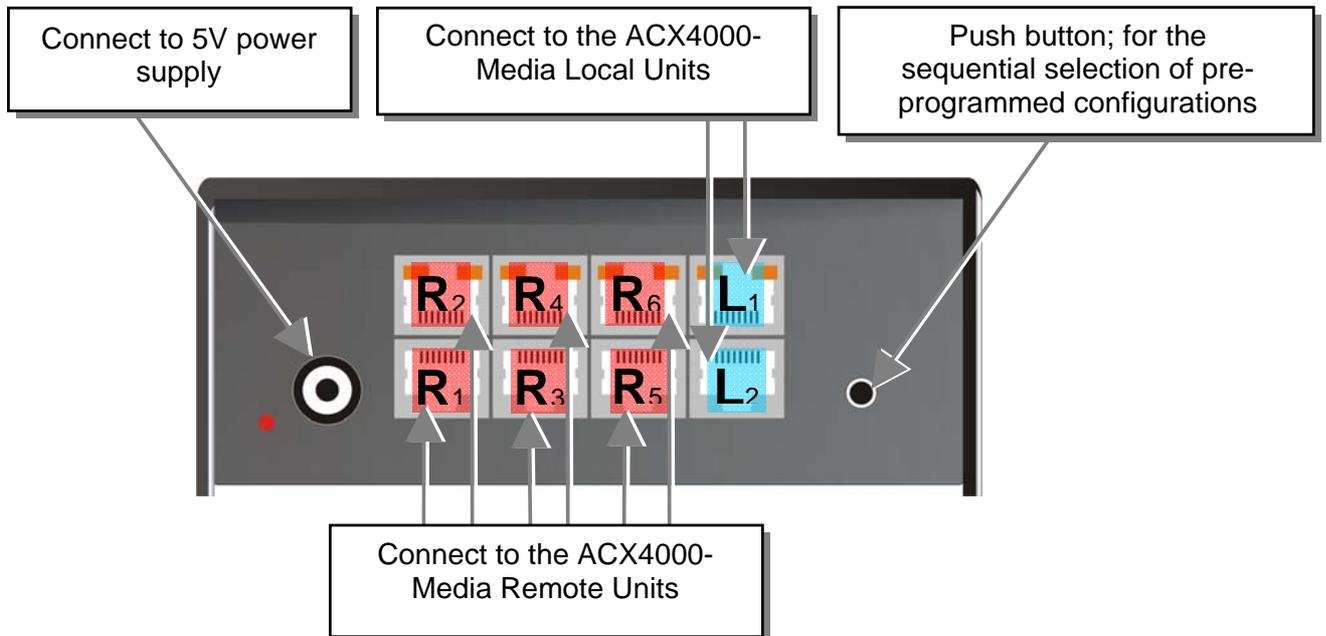
The signals of 2 Local Units is switched on up to 6 outputs and transferred over CATx- cables to 6 Remote Units. Optionally, a further ACX4000 Switch can be inserted for a second switching stage.
