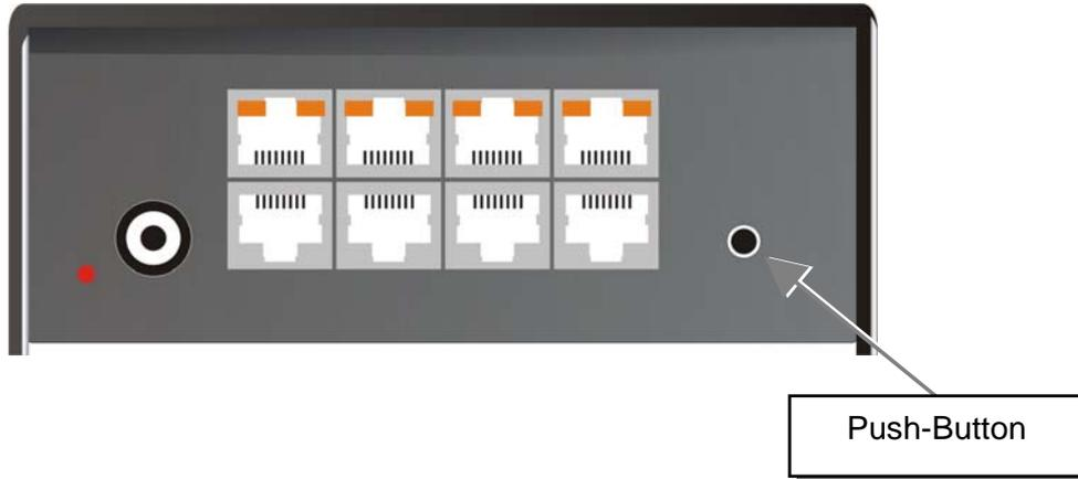
With each key press, the next macro stored in the device is called and the programmed switching configuration is loaded. The macro will only be executed if the push button is not operated for longer than 2 seconds. With the first key press, the macro display is switched on. The LED with the number of the active selected macro flashes. With each key press, the display will switch to the next LED. The selection of a not (yet) programmed macro will be interpreted as a reset (see below).
