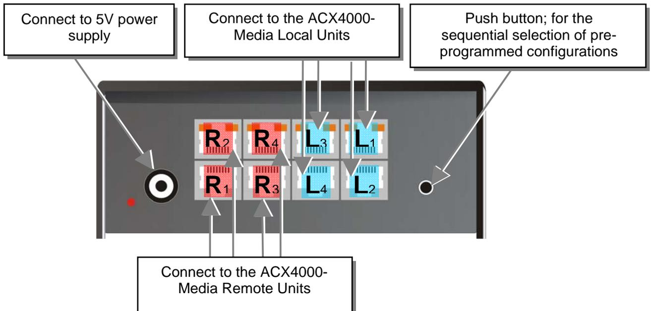
The signals of 4 Local Units is switched on up to 4 outputs and transferred over CATx- cables to 4 Remote Units. Optionally a further ACX4000 Switch can be inserted for a second switching stage.
