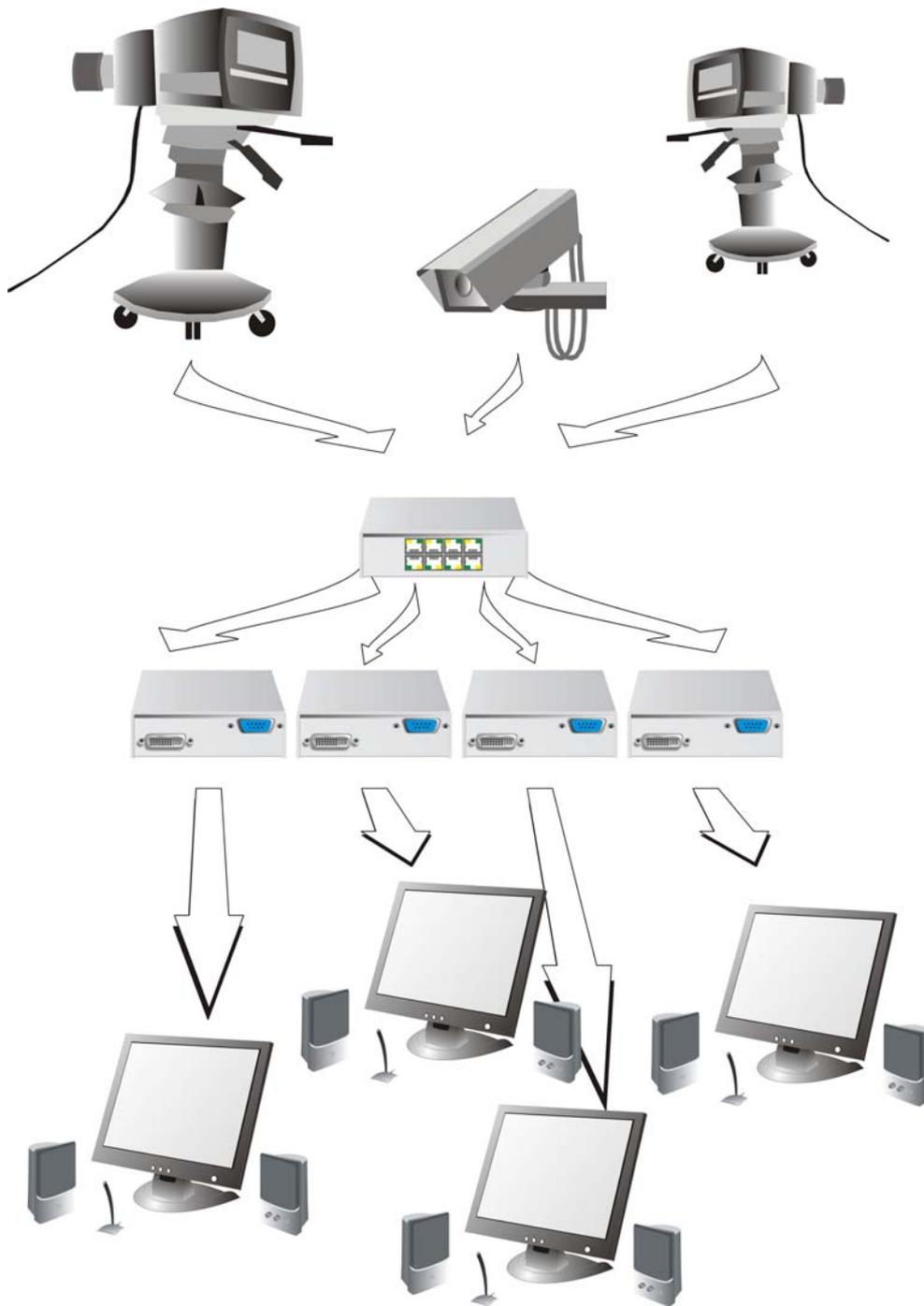
**Three video sources are switched over the ACX4000 Switch on four different screens.**
