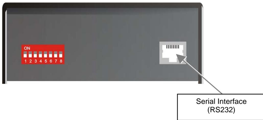
You can find the allocation of the serial interface under “**Serial Interface (external switchbox) DCE**” on page **103**. A standard cable RJ45 / DB9 to the CPU is included in delivery.
