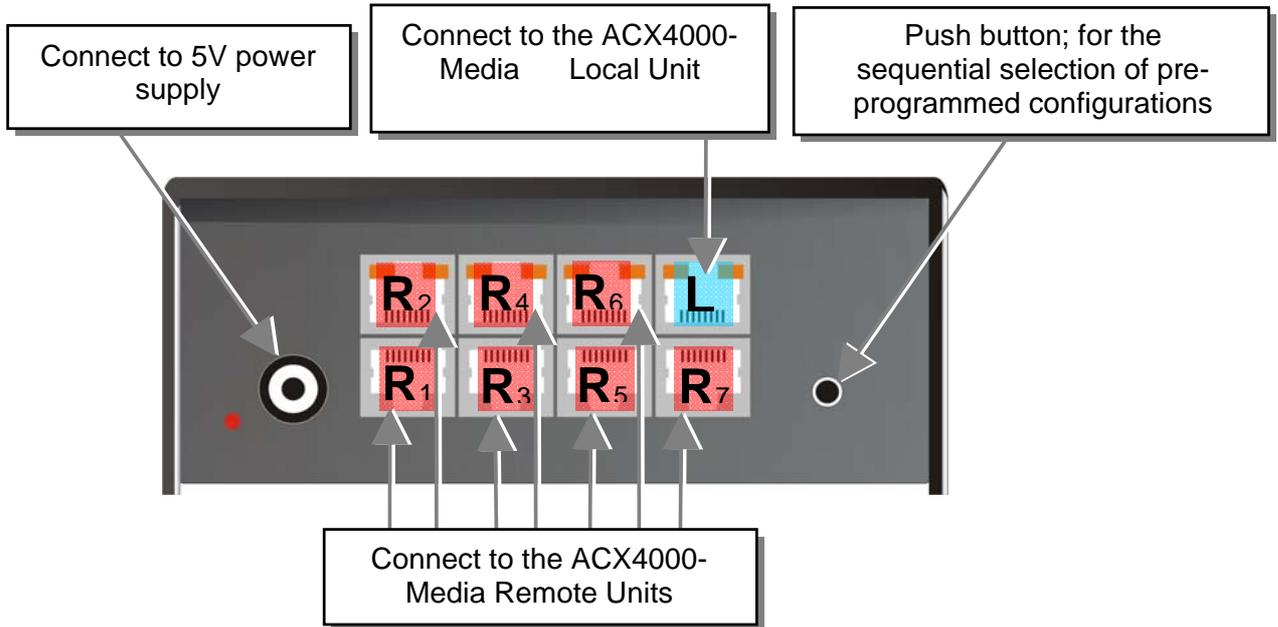
The signal of a Local Unit is switched on up to 7 outputs and transmitted over CATx- cables on up to 7 Remote Units. Optionally a further ACX4000 Switch can be inserted for a second switching stage.
