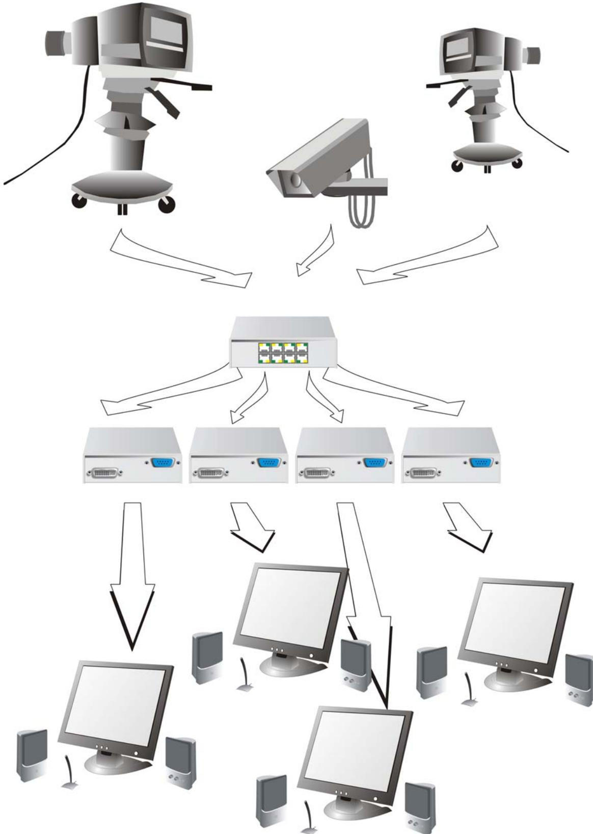
**ACX4000 as Cross point- Switch (here: 3x Input/ 4x Output)**
