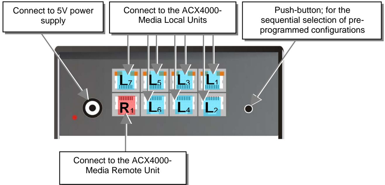
The signals of 7 Local Units can be switched to one output and be transferred over CATx-cables to one Remote Unit. Optionally a further ACX4000 Switch can be inserted for a second switching stage.
