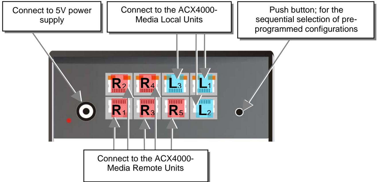
The signals of 3 Local Units is switched on up to 5 outputs and transferred over CATx- cables to 5 Remote Units. Optionally a further ACX4000 Switch can be inserted for a second switching stage.
