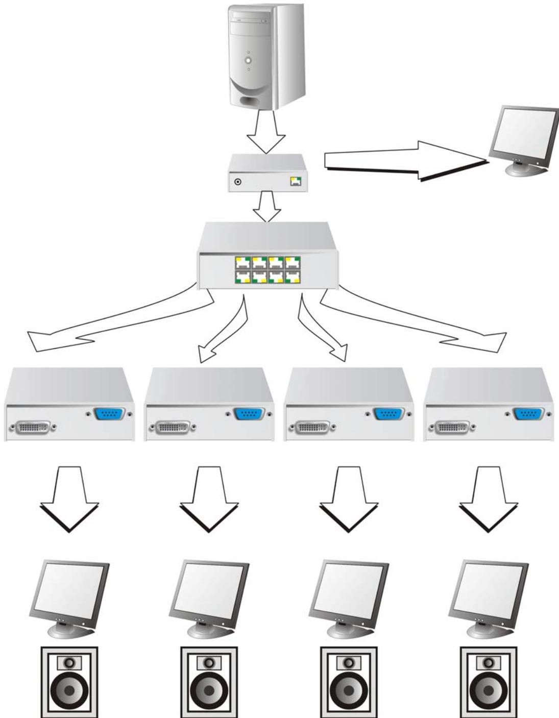
**A video/audio source is switched over the ACX4000 Switch to 4 different screens/loudspeakers. Additionally a control monitor can be attached at the Local Unit.**
