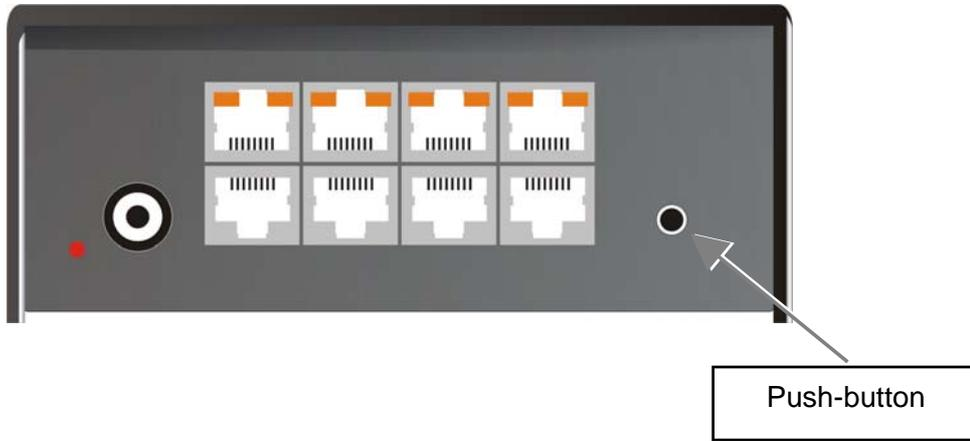
The device switches to the next channel with each key press. The changeover will only be executed if the push-button is not operated for longer than 2 seconds. With each key press, the display will switch to the next channel as indicated by a rapidly blinking LED. If the last channel is reached, the device will cycle to the first channel.
