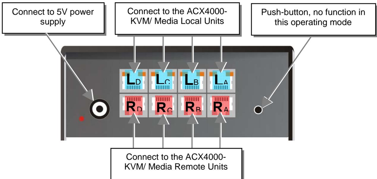
Four different signals from four Local Units are transferred over CATx- cables to one equivalent Remote Unit. This allows an extension to the cable length, if the usual 140m distance by CATx- cables is not sufficient.
