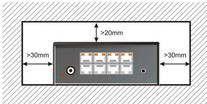
If mounted into 19" racks: the space to the left and to the right side of the ACX4000 must kept free!
