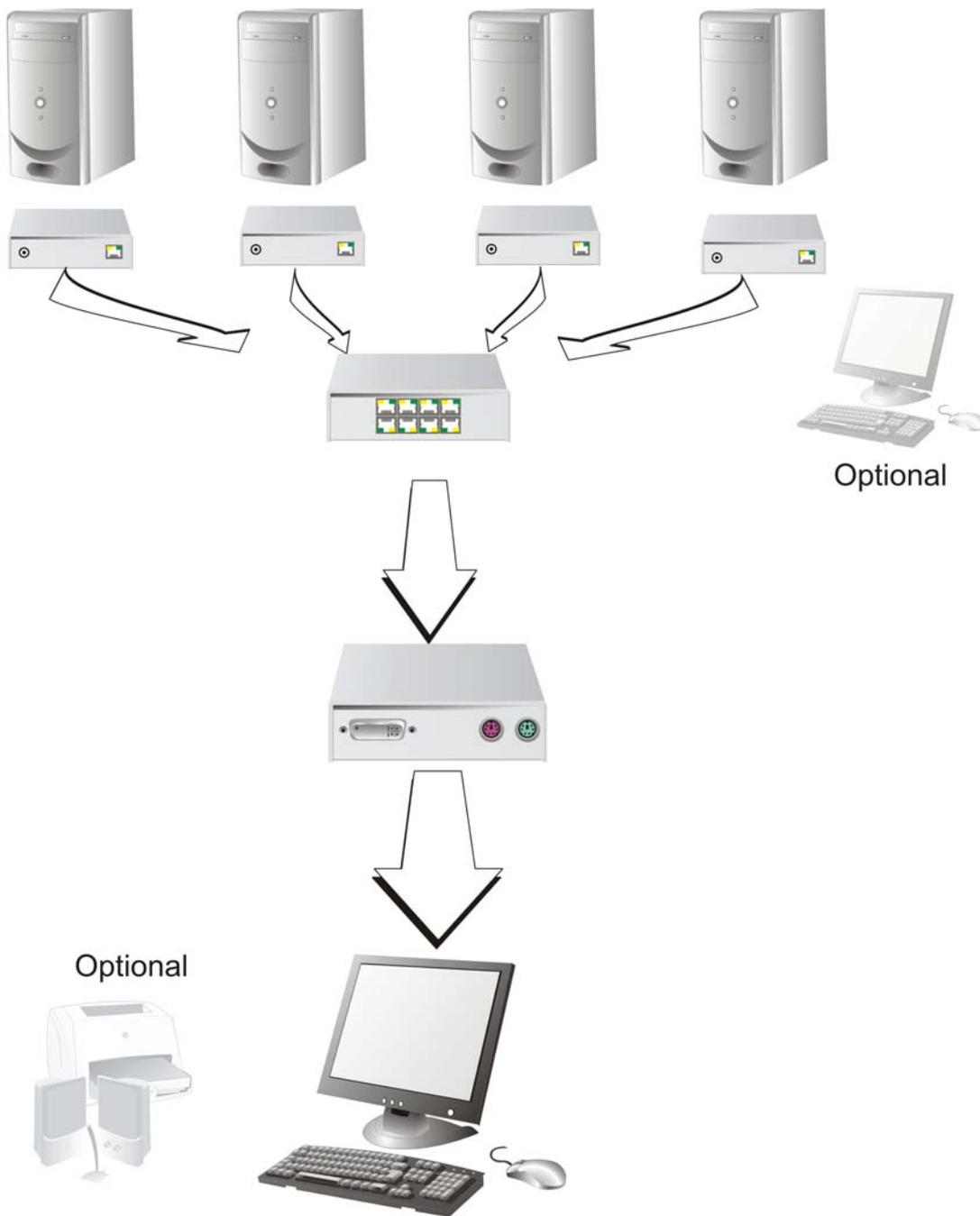
**Four CPUs are switched over the ACX4000 Switch to one console.**
