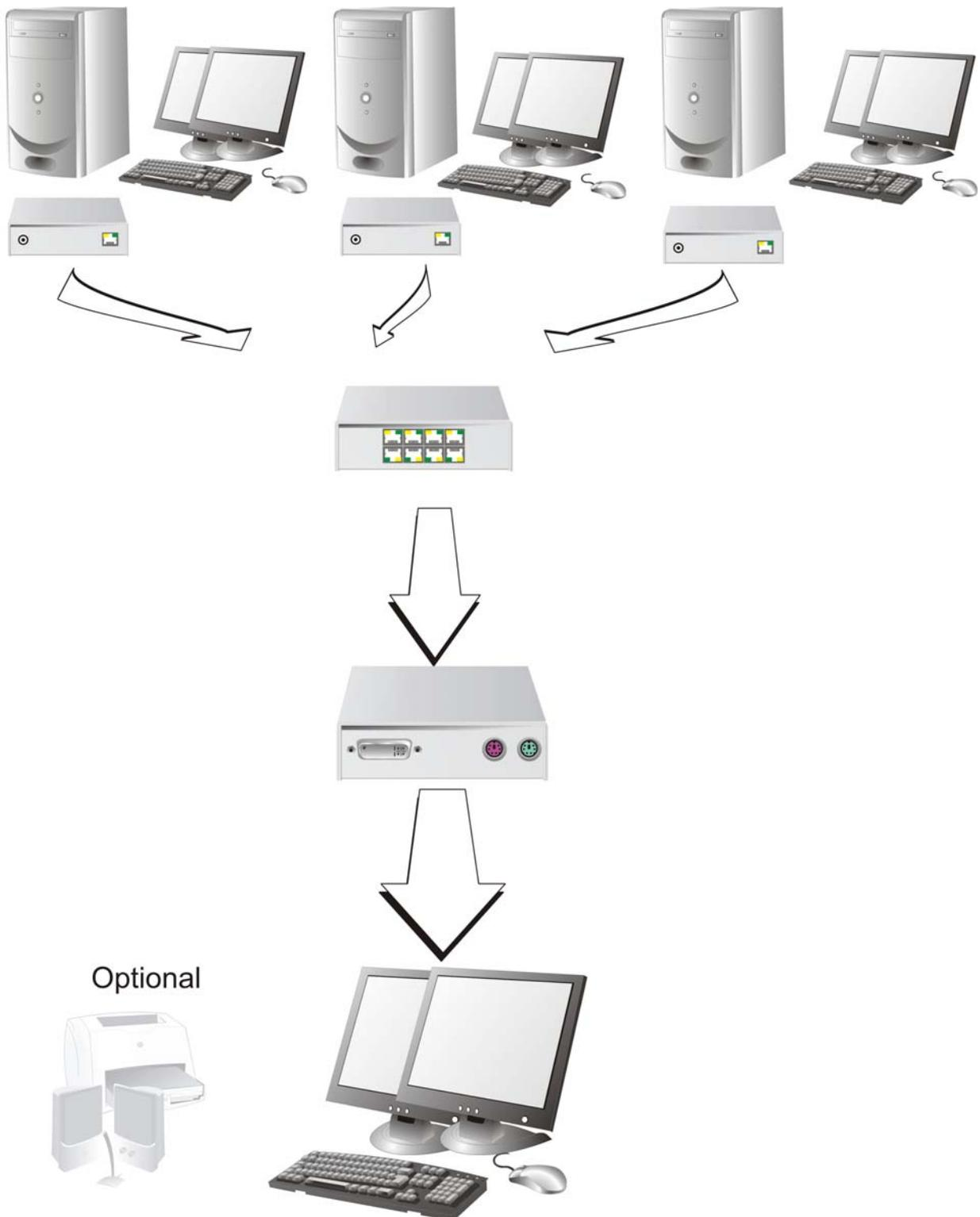
**Three CPUs with dual head graphic cards and local consoles switched over the ACX4000 Switch to one console.**
