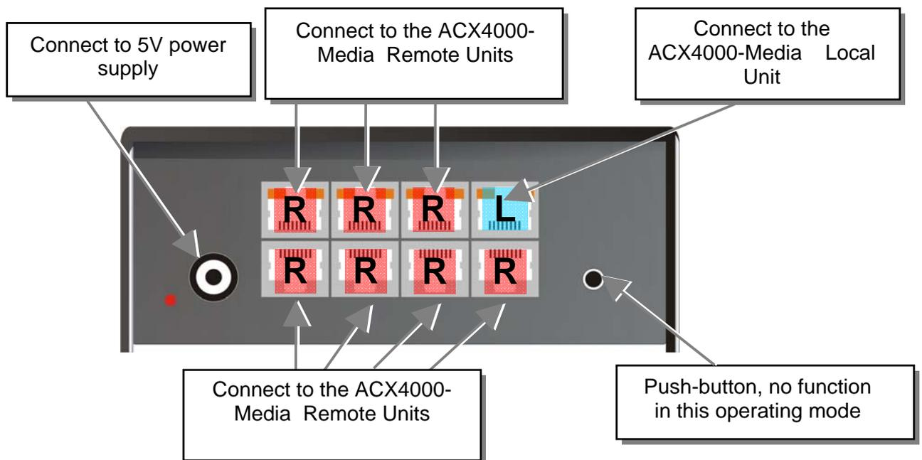
A single signal from a Local Unit is distributed on up to 7 outputs and transferred over CATx- cables on up to 7 Remote Units. Using a second stage of Multiplex Repeaters up to 49 monitors can be supplied with video (and optionally audio).
