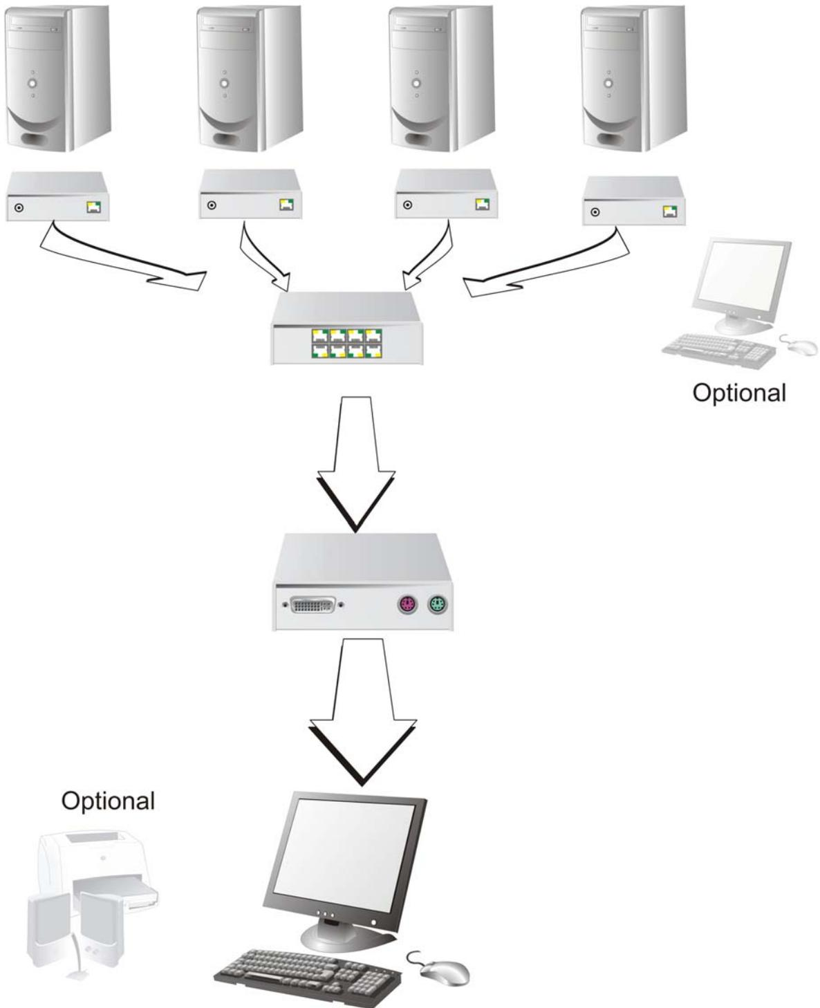
**ACX4000 as Single head KVM- Switch (to 7:1) optional with a local console and/ or serial/ audio option**
