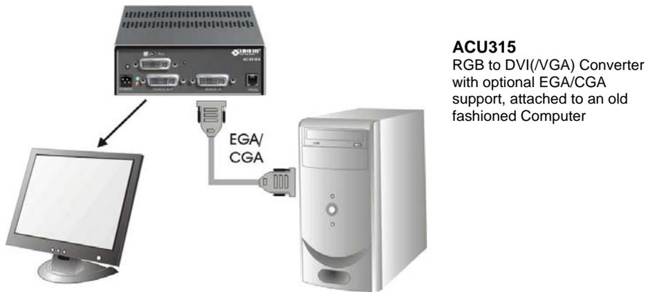
**Figure 19** ACU315A Converter with optional EGA/CGA support, attached to an old fashioned Computer
