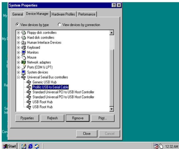
Setup9. Back to the system properties and make sure “Prolific USB-to-Serial Cable” show in the screen.
