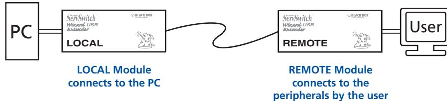
Hence, the LOCAL module connects directly to the system, while the REMOTE is at the other end of the twisted pair cable(s) and attaches to the video monitor, USB peripherals and sound equipment.
