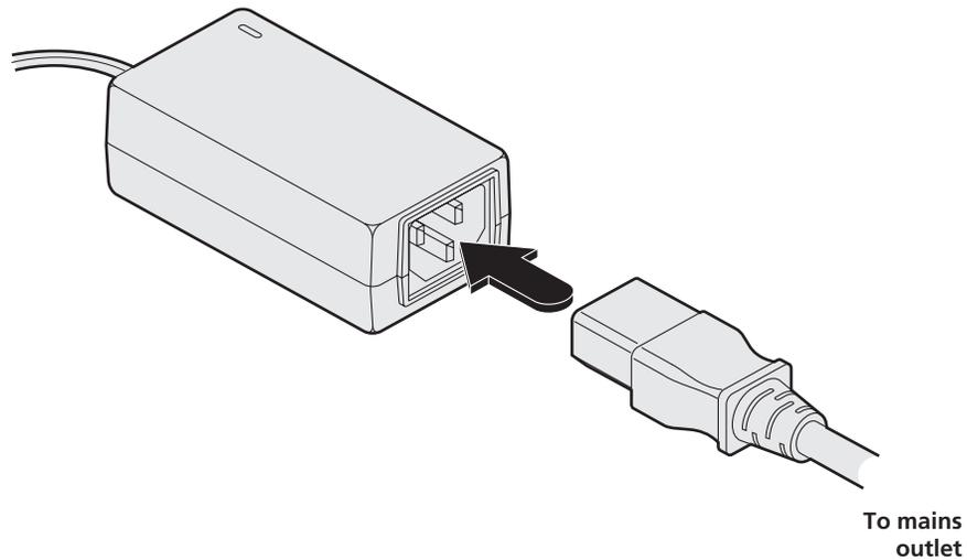
Figure 3-12. Attaching the power cord to the adapter
