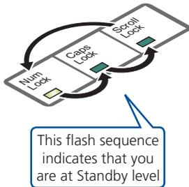
The indicators on the keyboard linked to the remote unit will begin to flash in sequence. Also, the green indicator adjacent to the CATx link socket will flash.
