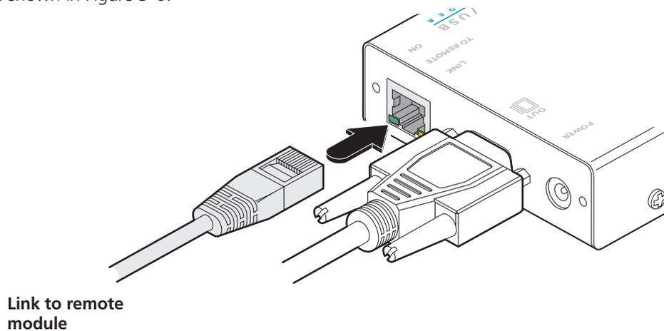
Figure 3-6. Attaching the CATx link cable
