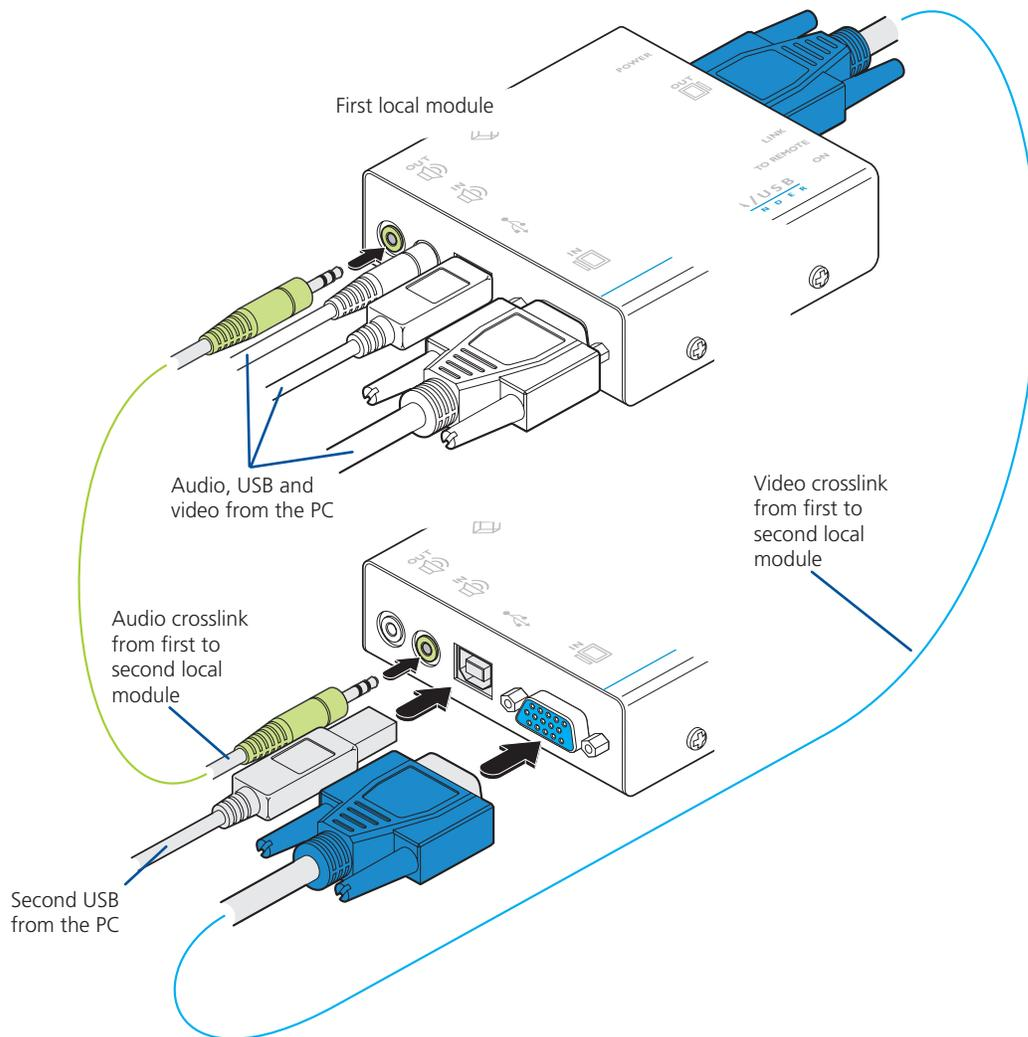
Figure 3-14. Interconnections required for a dual user configuration
