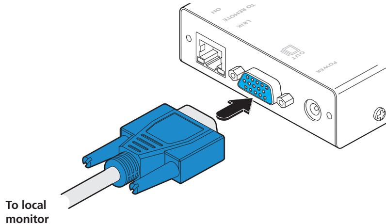
Figure 3-5. Optionally attaching a local video monitor
