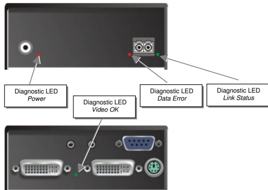
Diagnostic - LEDs at DVI-D KVM Extender
