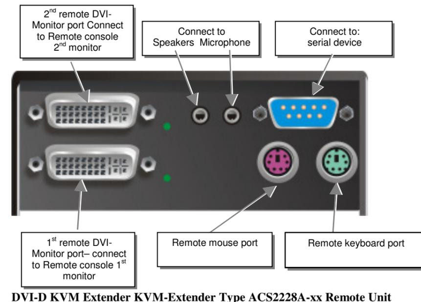
DVI-D KVM Extender KVM-Extender Type ACS2228A-xx Remote Unit
