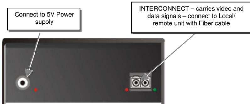
DVI-D KVM Extender KVM-Extender Type ACS2028A-xx Local/ Remote Unit
