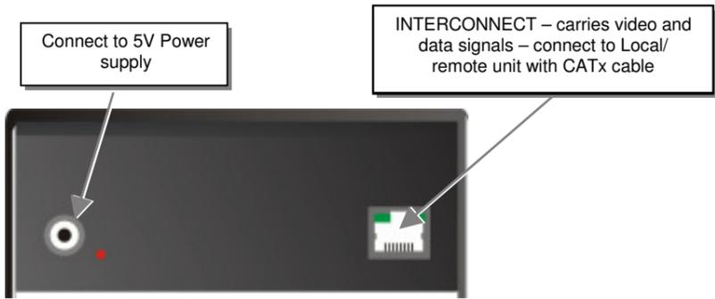
DVI-D KVM Extender KVM-Extender Type ACS2028A Local/ Remote Unit
