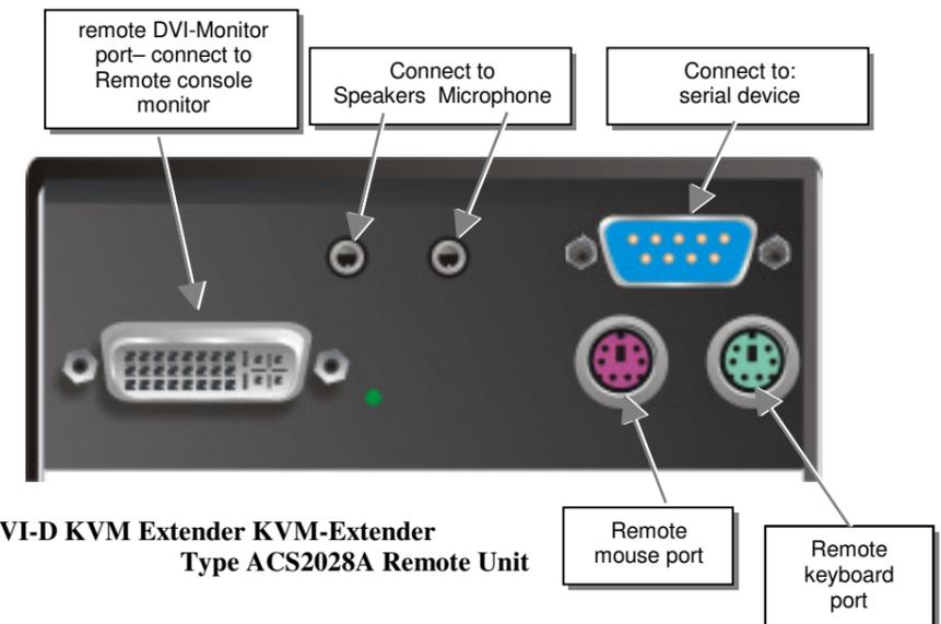
DDVI-D KVM Extender KVM-Extender Type ACS2028A Remote Unit
