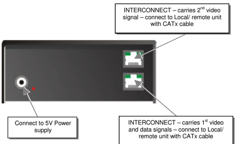
DVI-D KVM Extender KVM-Extender Type ACS2228A Local/ Remote Unit
