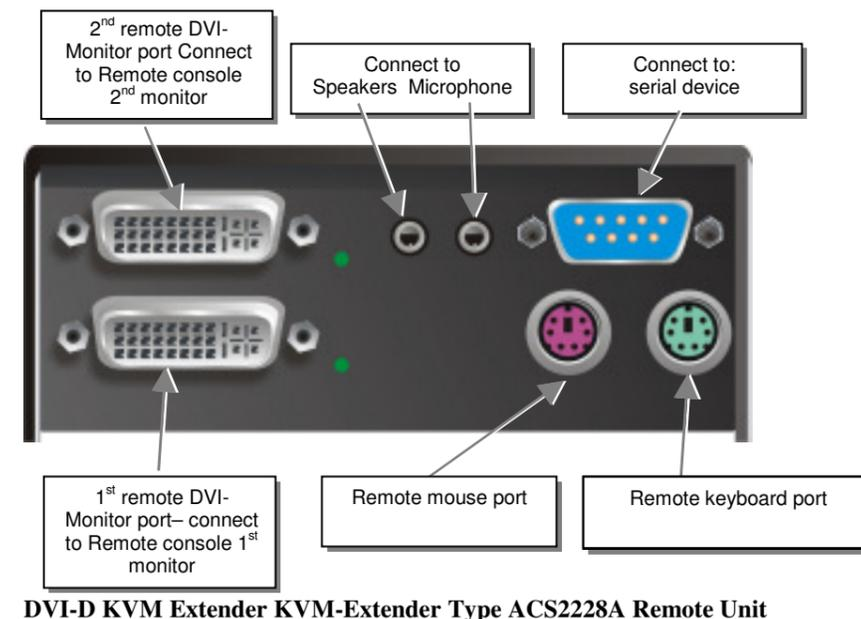
DVI-D KVM Extender KVM-Extender Type ACS2228A Remote Unit
