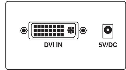
Figure 2. Local unit front view: DVI In port, power jack
