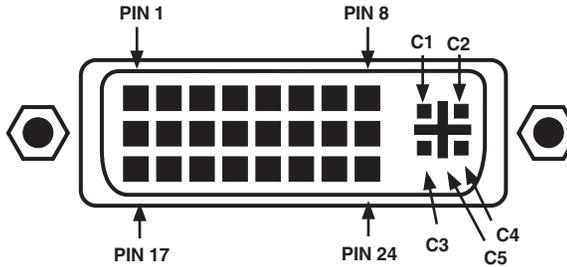
Figure 1. DVI-D connector pinning.
