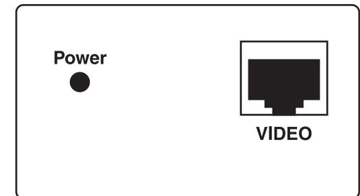
Figure 5. Remote unit rear view: Power LED, CAT5 port
