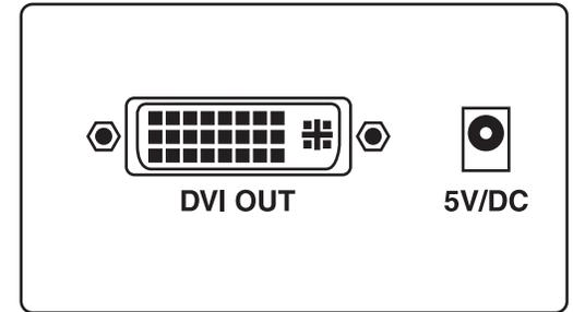
Figure 4. Remote unit front view: DVI Out port, power jack
