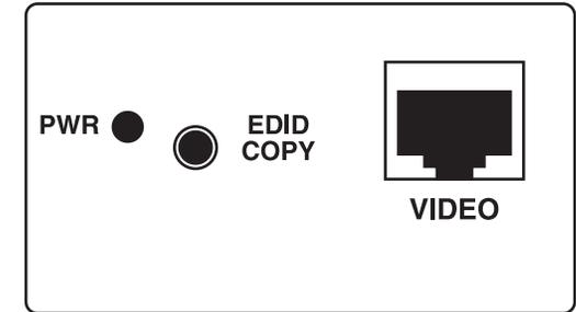
Figure 3. Local unit rear view: Power LED, EDID COPY button, CAT5 port
