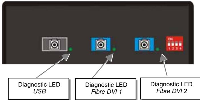
**Diagnostic LEDs at the ACS1xxA – Extender (Fibre Sockets)**
