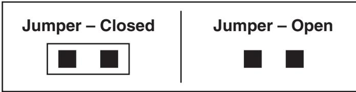
**Figure 6-9. Jumper closed and open.**
