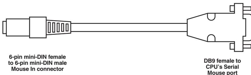
Figure 5-14. The Mouse adapter cable.
