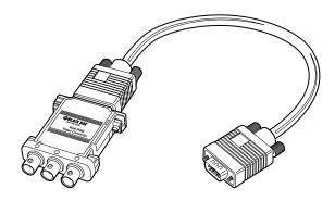
The VGA to RGB Video Converter is designed to take standard VGA-compatible video signals (incuding separate horizontal and vertical sync, as output by a computer or other device with an HD15 connector) and convert them to RGsB video signals (including composite sync on green, to be input by a monitor or other device with three BNC connectors).
