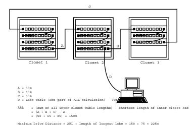
Once you have worked out the ARL and Maximum drive distance for your Network, you can use one of the two following tables to work out whether or not it falls within specification. Simply add up the number of MAUs and wiring closets on your network and cross-reference it against one of these two charts:
