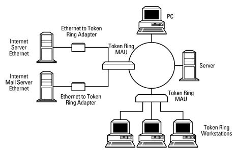
You can use the Ethernet to Token Ring Adapter to connect all types of Ethernet devices—including scanners, printers, and servers—to Token Ring networks.
