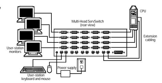
NOTE: For clarity, only one CPU is shown. Also, though separate extension cables are shown here, we recommend that you use our special Premium KVM CPU Cable (EHN408) to connect your CPU's first video port and its keyboard and mouse ports to the Switch. This cable has a central video strand with keyboard and mouse strands bonded to either side.
