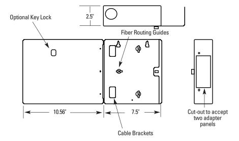
The Fibre Wall Cabinet (JPM401A) accepts a mix of four adapter panels.
