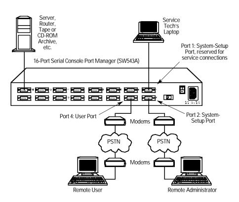
the Serial Console Port Manager, run a DB9 cable between the two. **Easy to configure, manage, and monitor.**
