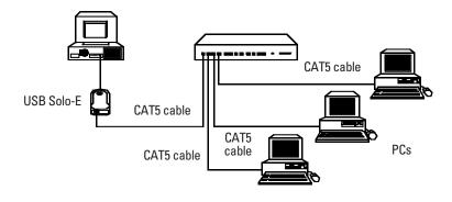
Link your USB devices to a CAT5 twisted-pair Ethernet network.
